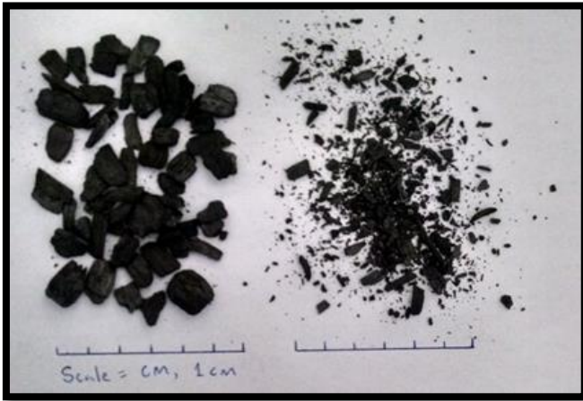
1: Large and Small Screened Fractions of Ecochar
